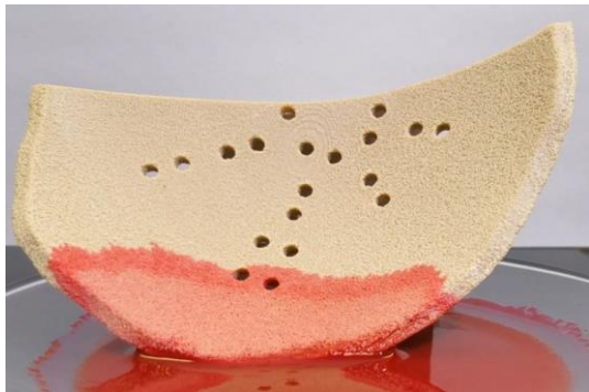
Figure 7: OsteoFab PEKK cranial implant section demonstrating vertical fluid conduction through the rough outer surface.
