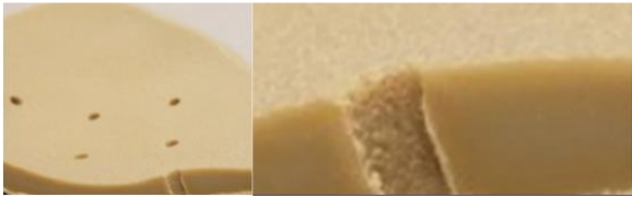
Figure 6: Cross section of a typical OsteoFab PEKK cranial implant, sectioned through one of the through holes. Note the fully dense part structure and visibly rough outer surface.
